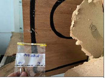
Photo 6 – Sample 509-HB-A, 2% asbestos containing black adhesive in the 109 building.
